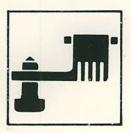
This warns that the dresser arm is in the raised position. When the dresser arm is raised, the holder and grinding stone automatically moves to the starting position for dressing. When the arm is lowered, the machine returns to the normal starting position.
