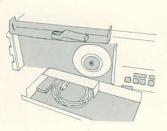
5. Check that the grinding stones have no defects and install one of them firmly.
